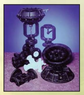
This all-plastic control valve for high-pressure fluids is completely corrosion resistant and reduces weight by more than 50% over metal versions. All the black components, including the bonnet, pneumatic actuator, and T-intersection, are molded with an RTP 4000 Series reinforced PPA compound. The shell and core design provides tremendous strength and impact resistance while preventing the white PTFE parts from creeping under excessive temperatures and pressure.
